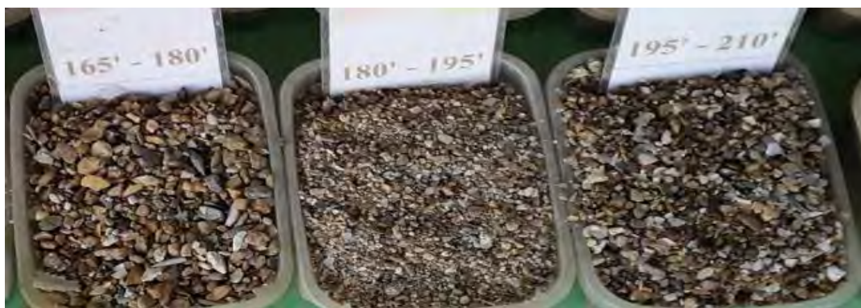
Photo 67: Alluvium Lithological Variation in Zay Village Tubewell, Pone Hnyat Village Tract, Myittha (50 to 64 m), Nov. 2016
