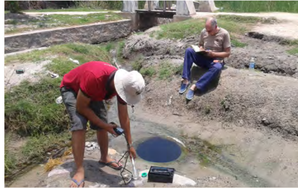
Photo 52: Measuring Temperature and Salinity in Hot Springs
