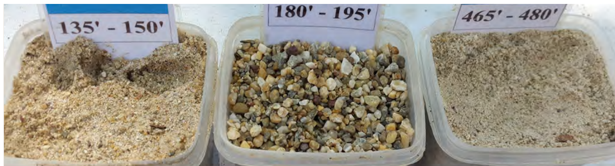
Photo 31: Lithological Variation in Kyauksauk Village TW, Irrawaddy Formation (41-46, 55-60, 142-146 m), Pakokku Syncline
