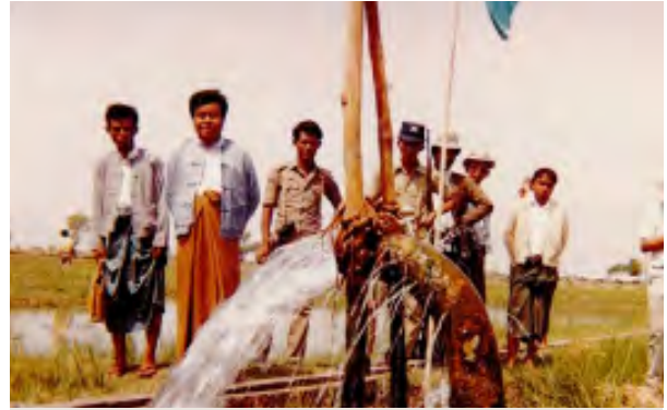
Photo 37: Uncontrolled Flow from Rusted Tubewell, Lengauk
