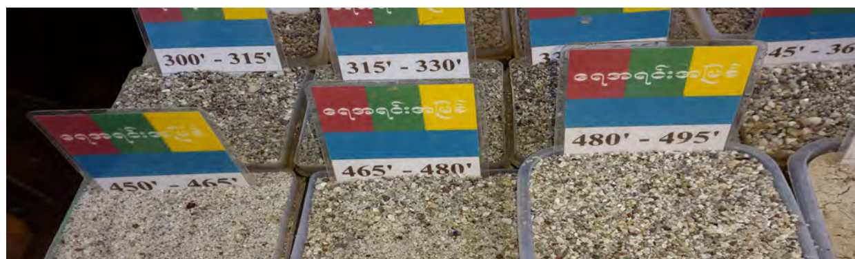
Photo 43: Coarse Sand and Fine Gravel from Twin Taw Village Tubewell, Irrawaddy Formation (137- 181 m)
