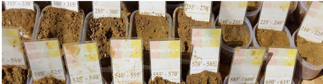
Photo 26: Taungbyin (2) Ward, Taungdwingyi. Yellow/Brown Clayey/Silty Sand Aquifer (165-175 m), Nov 2016
