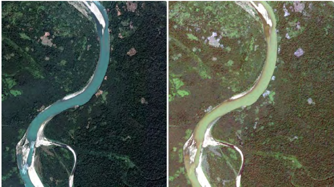
Figure 13: VHR image (Pleiades), on the left vs HR image (Rapid Eye), on the right
