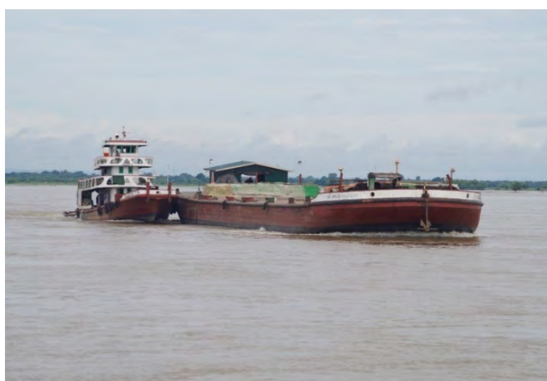
Figure 155 - Barge with partial load and push-tug
