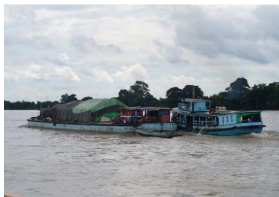
Figure 154 - Barge Carrying Rice, with Push-Tug on Starboard
